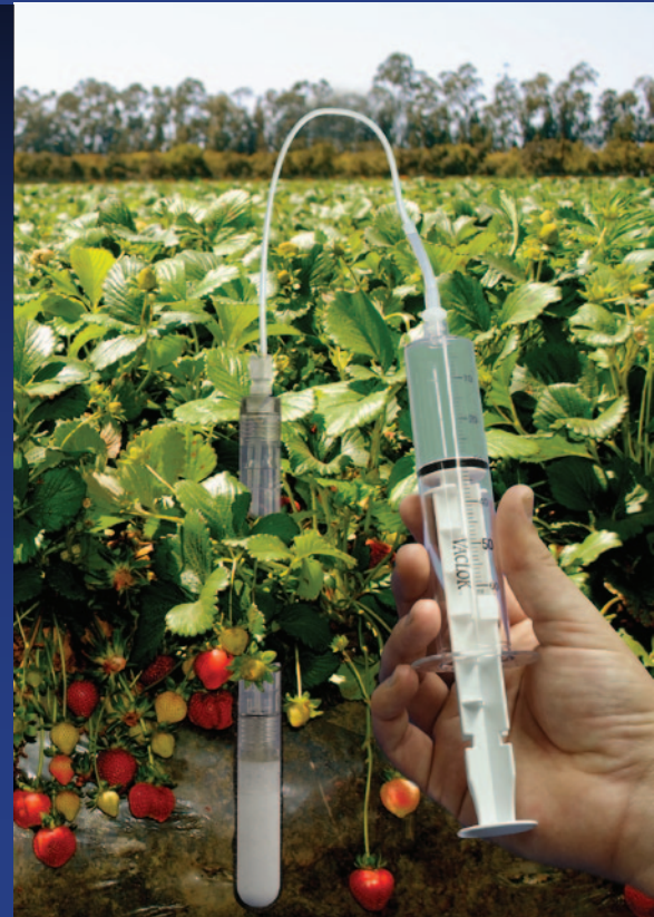
Figure 3. Using 1909L and 1930 to collect a pore water sample in a strawberry field. This sturdy sampler can be capped during the off-season, and then collected from quickly after watering events during the growing season!
