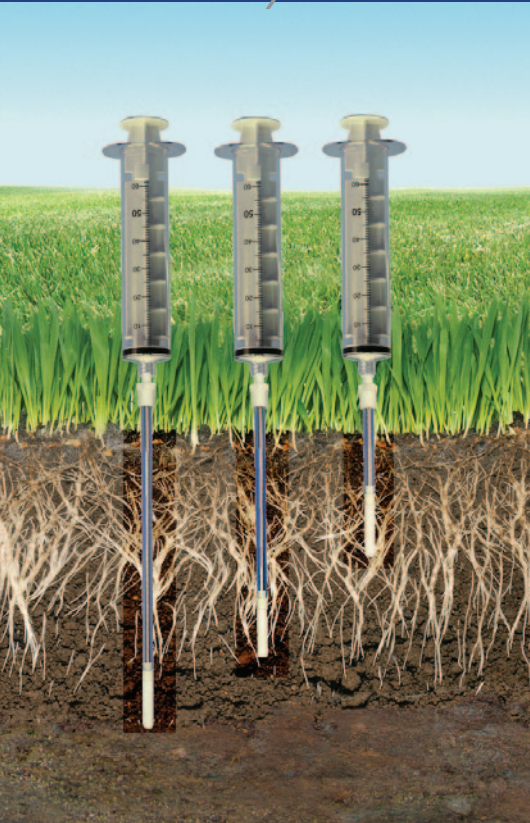
Figure 1. 1910LL installed to assess pore water in a turf zone. By creating minimal disturbance to native soils, these samplers offer greater reliability along with their mobility!
