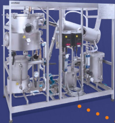
FT29 Batch Solvent Extraction & Desolventising Unit
