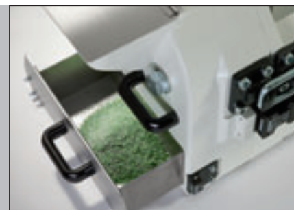
Grinding result with a gap width of 1 mm
