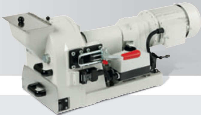
Filling of the funnel with pre-crushed glass bottles
