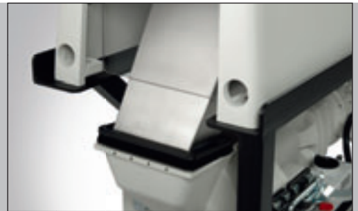
A connection chute automatically conveys the pre-crushed material onward for fine grinding.
