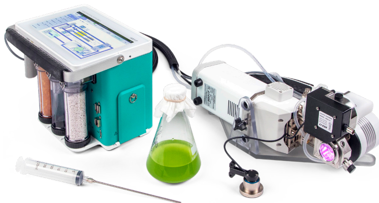
Figure 1. The aquatic chamber directly measures CO 2 assimilation by algae in suspension under controlled steady-state conditions. The LI-6800 console (left) provides a conditioned air supply, data file management, and the configuration interface. The LI-6800 sensor head (right) provides flow control valves, gas analyzers, and other sensors. The 6800-18 Aquatic Chamber with fluorometer (far right) holds a 15 mL aquatic sample.
