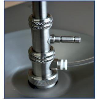
The assembly incorporates an automatic de-blocking device that prevents the jet nozzle from becoming blocked, the de-blocking needle is activated by an integral compressor.
