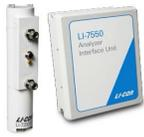
A high-speed, high-precision CO<sub>2</sub>/H<sub>2</sub>O gas analyzer combining the benefits of open and closed path gas analyzers for eddy covariance measurements. Includes LI-7550 Analyzer Interface Unit, SmartFlux<sup>®</sup> 2 System, head cable (5 m), serial cable and USB adapter, DAC, auxiliary input, SDM Cables (5 m), Ethernet cable (5 m), network switch, 16 GB industrial grade USB drives, instruction manual, Windows<sup>®</sup> Software, and EddyPro<sup>®</sup> Software.
