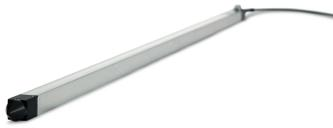
The LI-191R Line Quantum Sensor measures PAR (400-700 nm) using a 1-meter quartz rod connected to a housing containing a silicon photodiode and glass filters. Continuous photodiode rod integrates signal over entire 1-meter length. Available with 2-meter or 5-meter cable and BNC or SMV terminals. Includes a bubble level.
