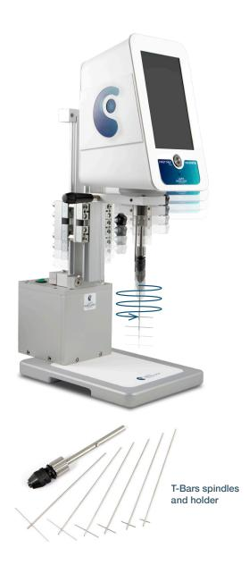
The HELIPRO device makes it possible to measure viscosity of gels, pastes, creams and more generally products that do not flowing.
