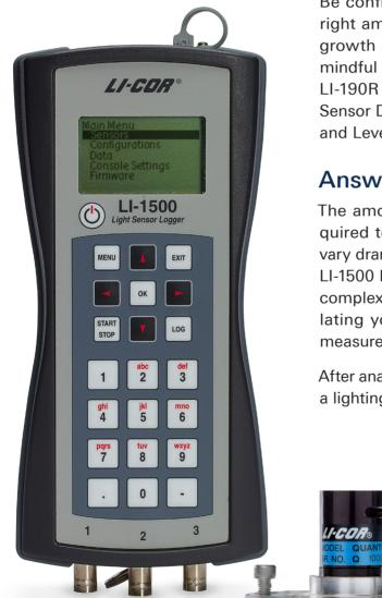
Be confident that you are providing the right amount of light for achieving ideal growth and maximum yield while being mindful of your bottom line. Includes the LI-190R Quantum Sensor, LI-1500 Light Sensor Data Logger, and 2003S Mounting and Leveling Fixture.
