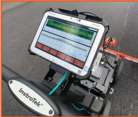
*The on-board computer displays density, compaction, a line graph, and a contour map of the measurements.*
