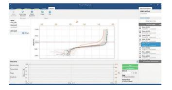
This software enables control of the Automated Micromanipulator and connected oxygen, pH or CO<sub>2</sub> meter. PreSens Profiling Studio allows complete control with several step zones, variable travel velocity and waiting times of the AM. It is database supported and offers multiple features from clear data organization and export, annotations, easy creation of profiling templates, to different analysis functions.
